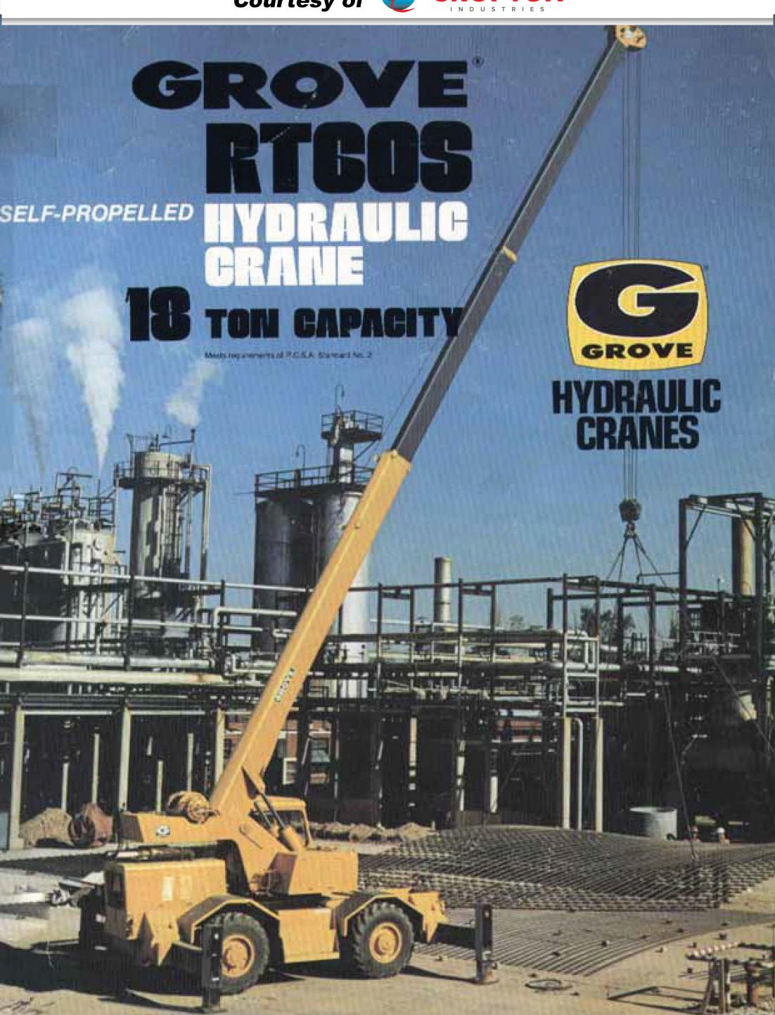
ROUGH TERRAIN MOBILITY . . . An automatic lockout is provided to prevent rear suspension system oscillation whenever the boom is in other than the forward position. An optional no-spin differential for the rear axle is also available. Rear axle and hydraulic pump disconnects provide more efficiency while traveling.
